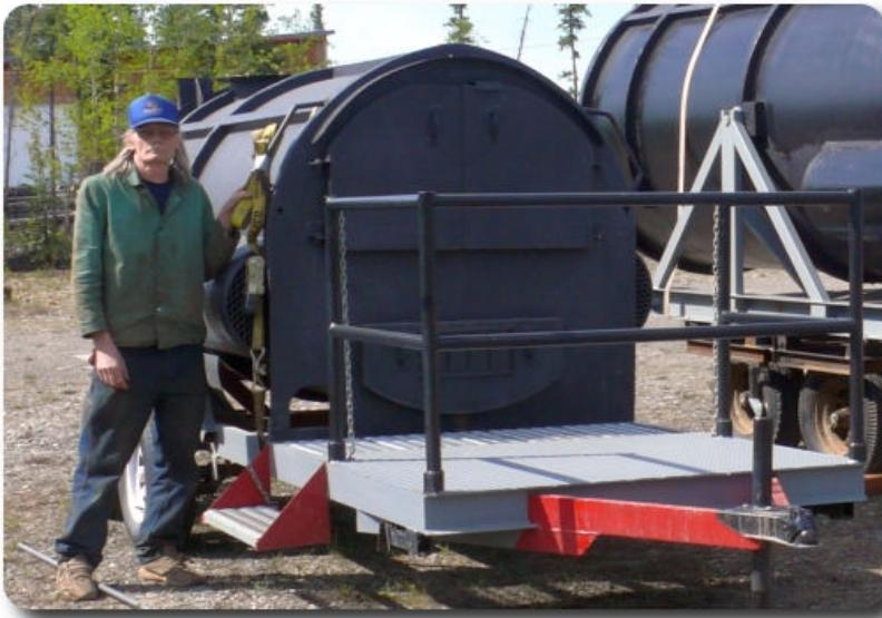
Once in Balance a Unit should stay in Balance for its entire life. The ash residue load will have a minimal effect on balance. The nature and design of the hinge/tipping feature is such that the ash load will be evenly distributed within the burn box, thus having no effect on tipping weight.
